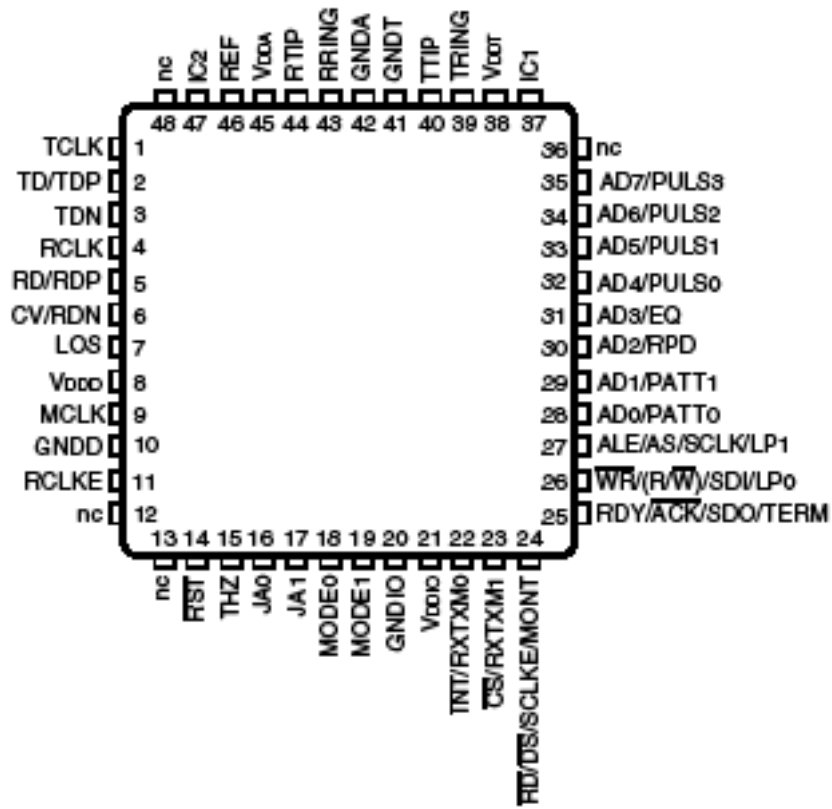
Figure-3 IDT82V2081 NLG Package Pin Assignment
