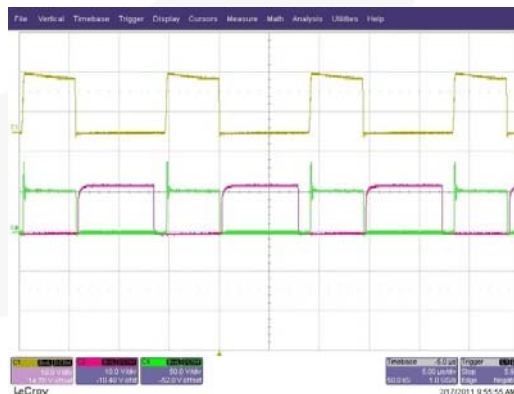
Figure 7. FAN6754WAMR+FAN6204MY, 115 V/60 Hz, 80% Load (Ch1: Gate, Ch2: Gate_SR, Ch4: V d5 )
