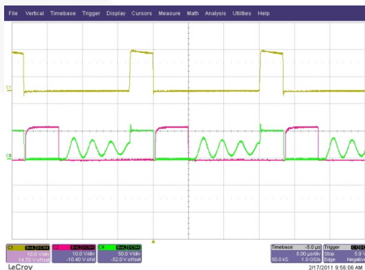
Figure 6. FAN6754WAMR+FAN6204MY 115 V/60 Hz, 20% Load (Ch1: Gate, Ch2: Gate_SR, Ch4: V d5 )
