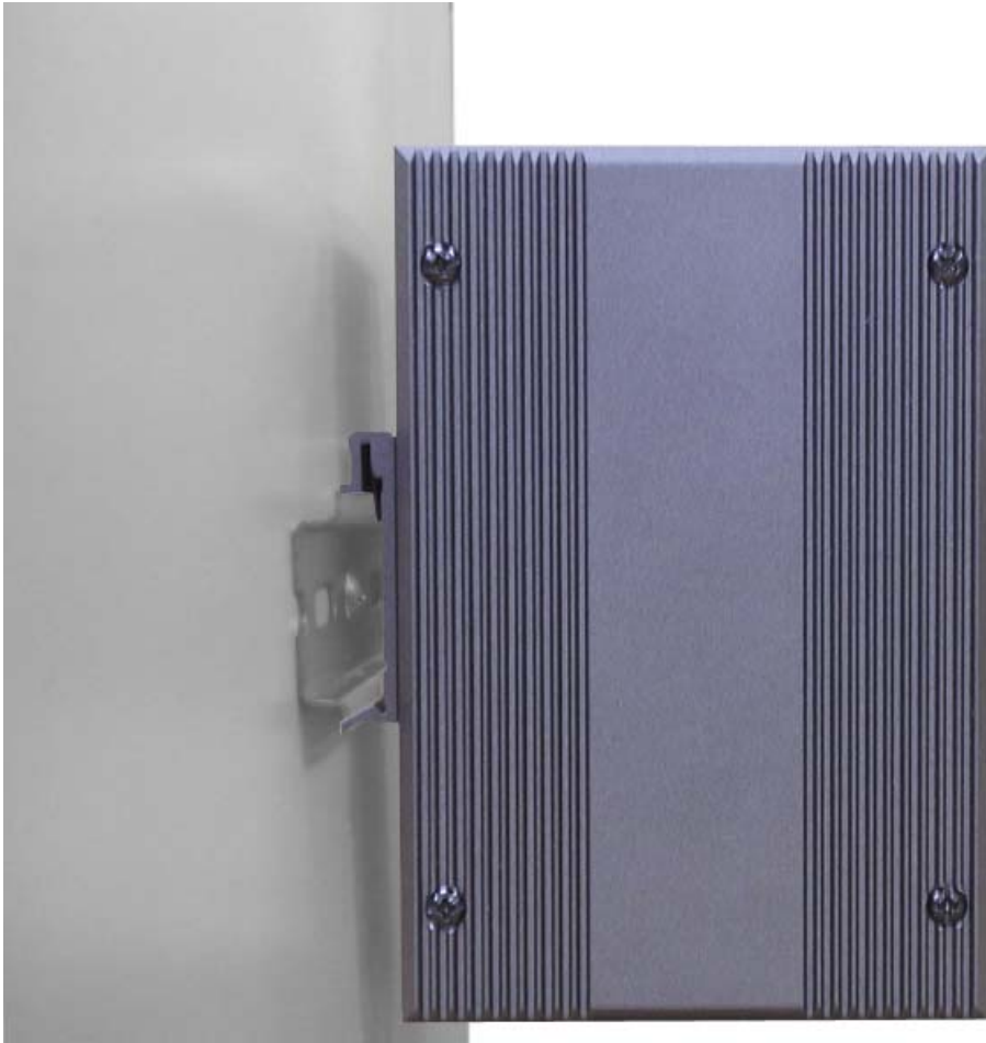
Figure 2.7: Installation to DIN-rail Step 2
