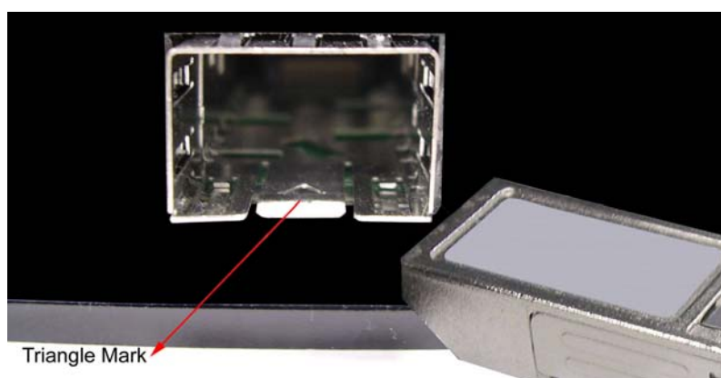
Figure 2.8: Transceiver to the SFP slot
