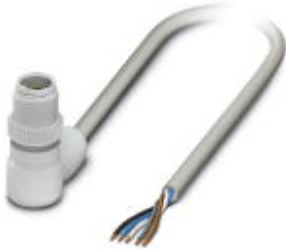
Sensor/Actuator cable, 5-position, PP-EPDM halogen-free, Gray RAL 7035, Plug angled M12, A-coded, on Free cable end, Cable length: 5 m, Hygienic design, with plastic knurl
