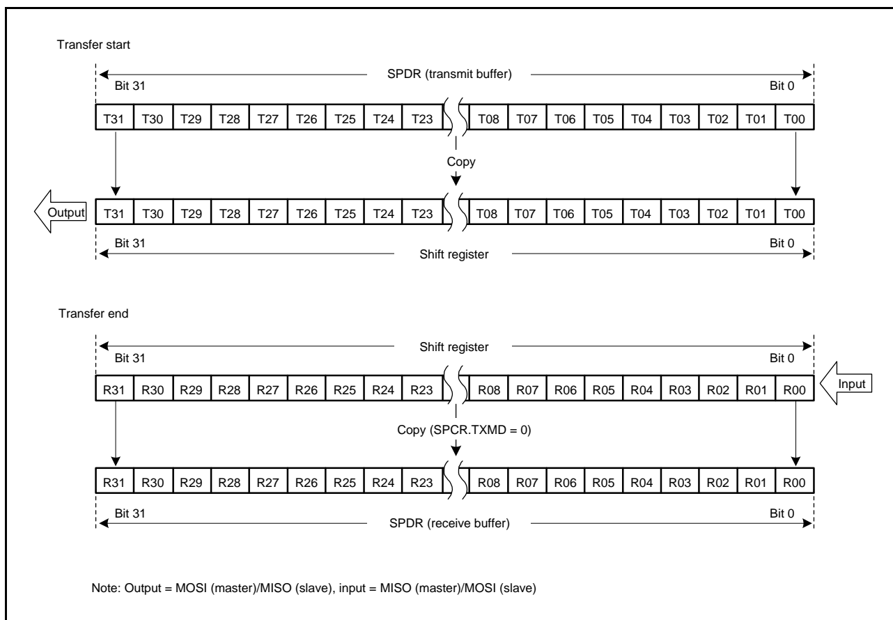
Figure 26.13 MSB First Transfer (1) (32-Bit Data, Parity Function Disabled)
