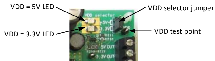
Figure 9. STEVAL-GLA001V1 evaluation board VDD selector components
