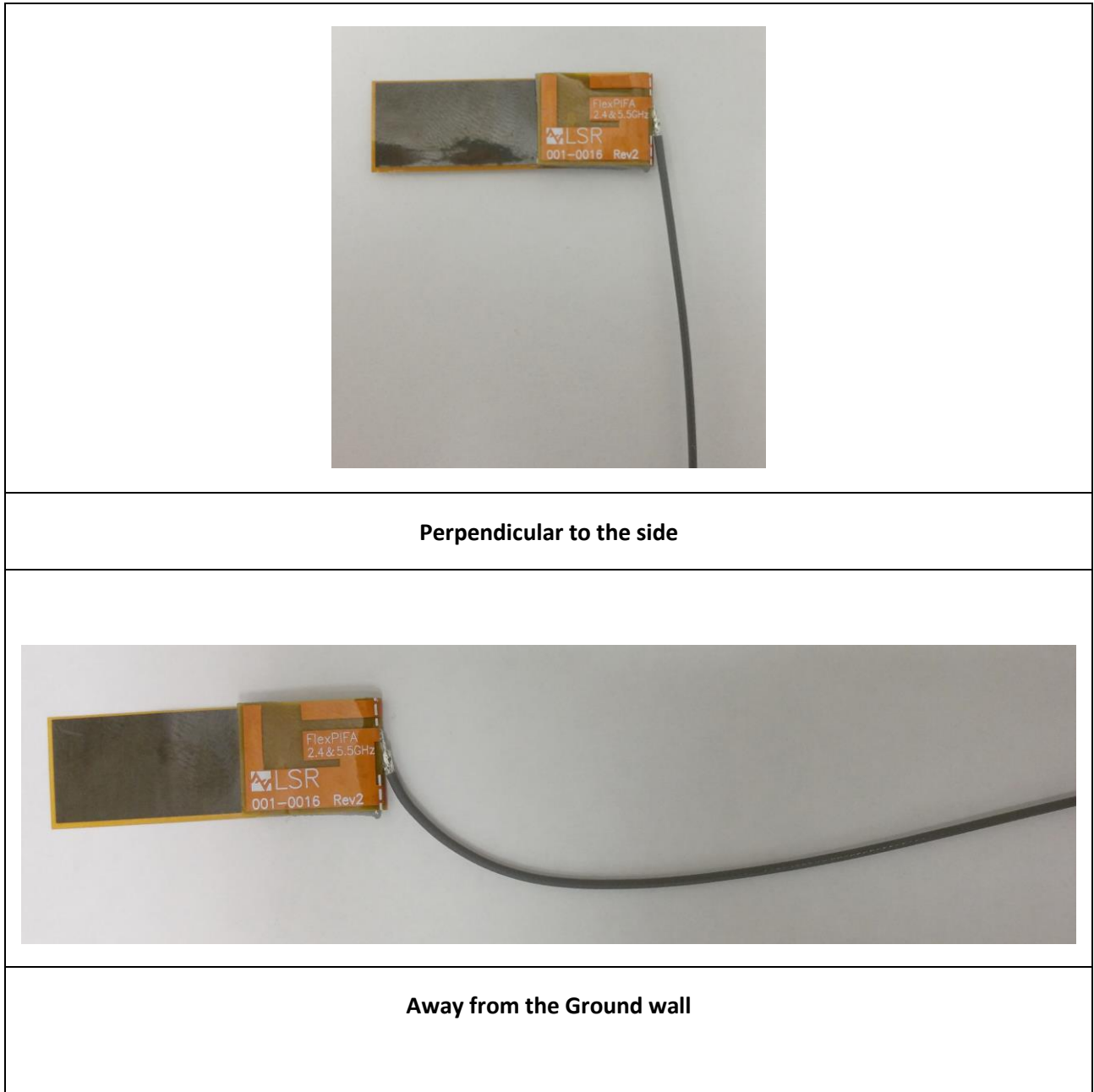
Figure 34 Recommended Cable Routing
