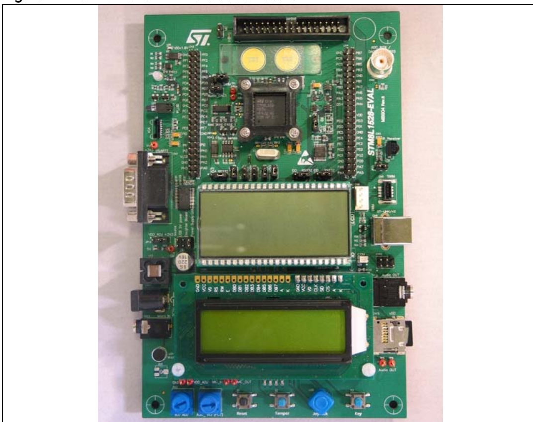
Figure 1. STM8L1528-EVAL evaluation board
