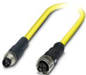
Sensor/Actuator cable, 3-position, PVC, yellow, Plug straight M8, on Socket straight M12 SPEEDCON, A-coded, Cable length: 1.5 m
