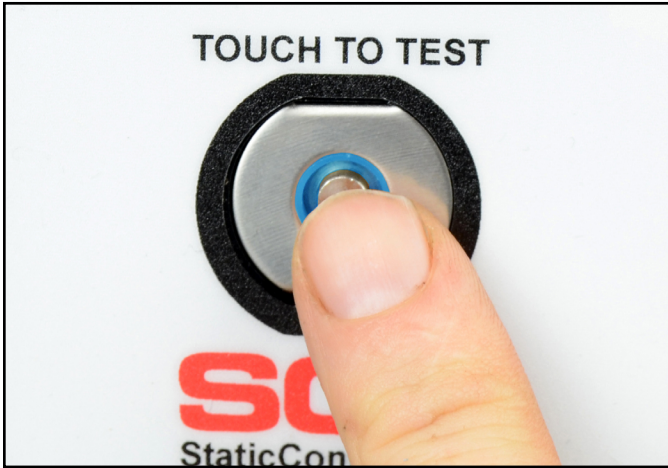
Figure 10. Bridging the test switch's contacts to initiate the test
