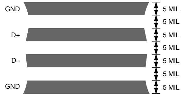
Figure 12. Typical Assignment of Signal Tracks
