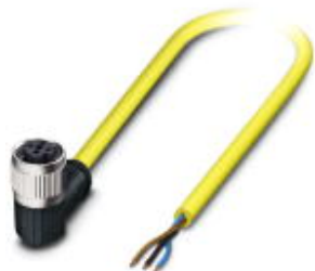
Sensor/actuator cable, 3-position, PVC, free cable end, on Socket angled M12 SPEEDCON, A-coded, cable length: 15 m
