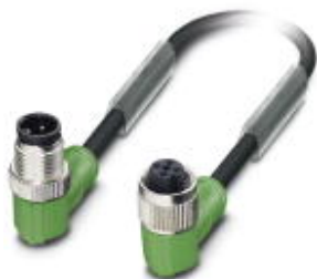
Sensor/actuator cable, 3-position, Variable cable type, Plug angled M12, A-coded, on Socket angled M12, A-coded, PIN 2+4 bridged, cable length: Free input (0.2 ... 40.0 m)
