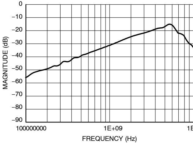
Figure 8. Differential Off Isolation
