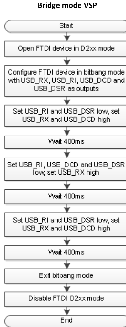
Figure 7: Flowchart for entering bridge mode VSP
