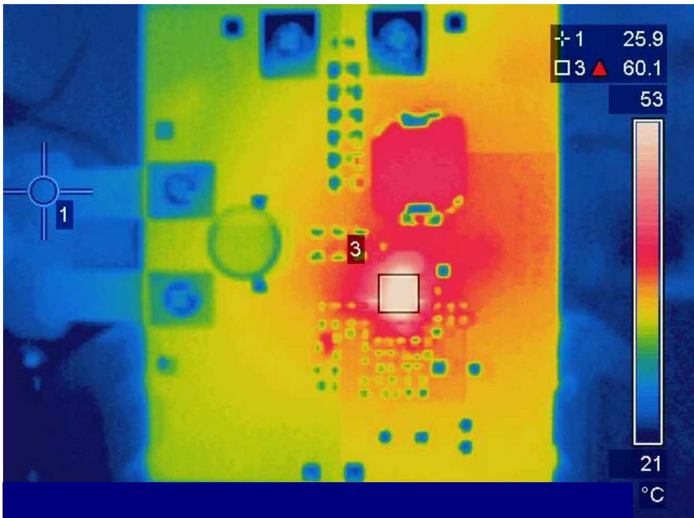
Fig. 17: Thermal Image at 6A load Test point 3 is IR3822A
