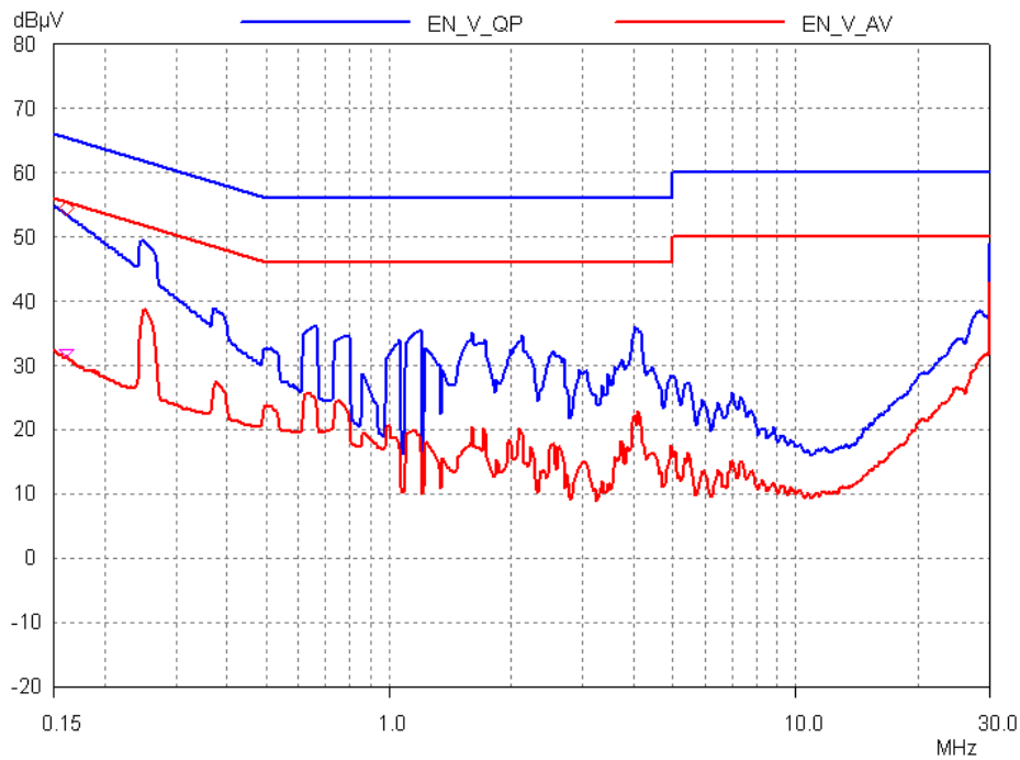
Figure 59 – Phase L1: Conducted EMI, Maximum Steady State Load, 230 VAC, 60 Hz, and EN55022 B Limits. Output Terminal Grounded
