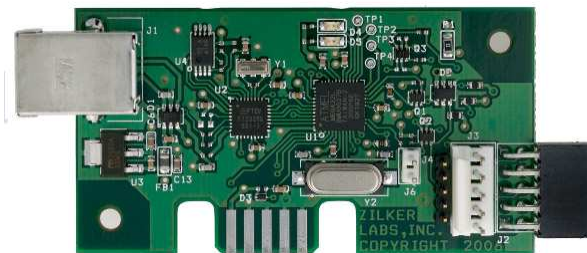
Figure 1. USB to SMBus Interface
