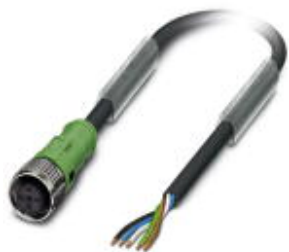
Sensor/actuator cable, 5-position, PUR halogen-free, black-gray RAL 7021, free cable end, on Socket straight M12 SPEEDCON, A-coded, cable length: 10 m
